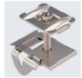
Connection clamp for fastening photovoltaic modules on support profiles of free-standing systems. Lockable pre-fastening of the module frames on the support profile. Suitable for slot width 10 mm. Lockable fastening of the PV module with Torx 30 wrench.
