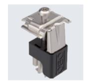
Universal clamp to mount photovoltaic modules on flat and pitched roofs, suitable as a clamp between 2 modules or as an end clamp. Lockable pre-fastening on TP 45 support profile and on STK and STL supports. Suitable for 10 mm slot width. Can be rotated through 90° after engaging. Lockable fastening of the PV module with Torx 30 wrench.
