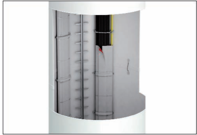
Bandaged rising section in the tower of a wind power plant
