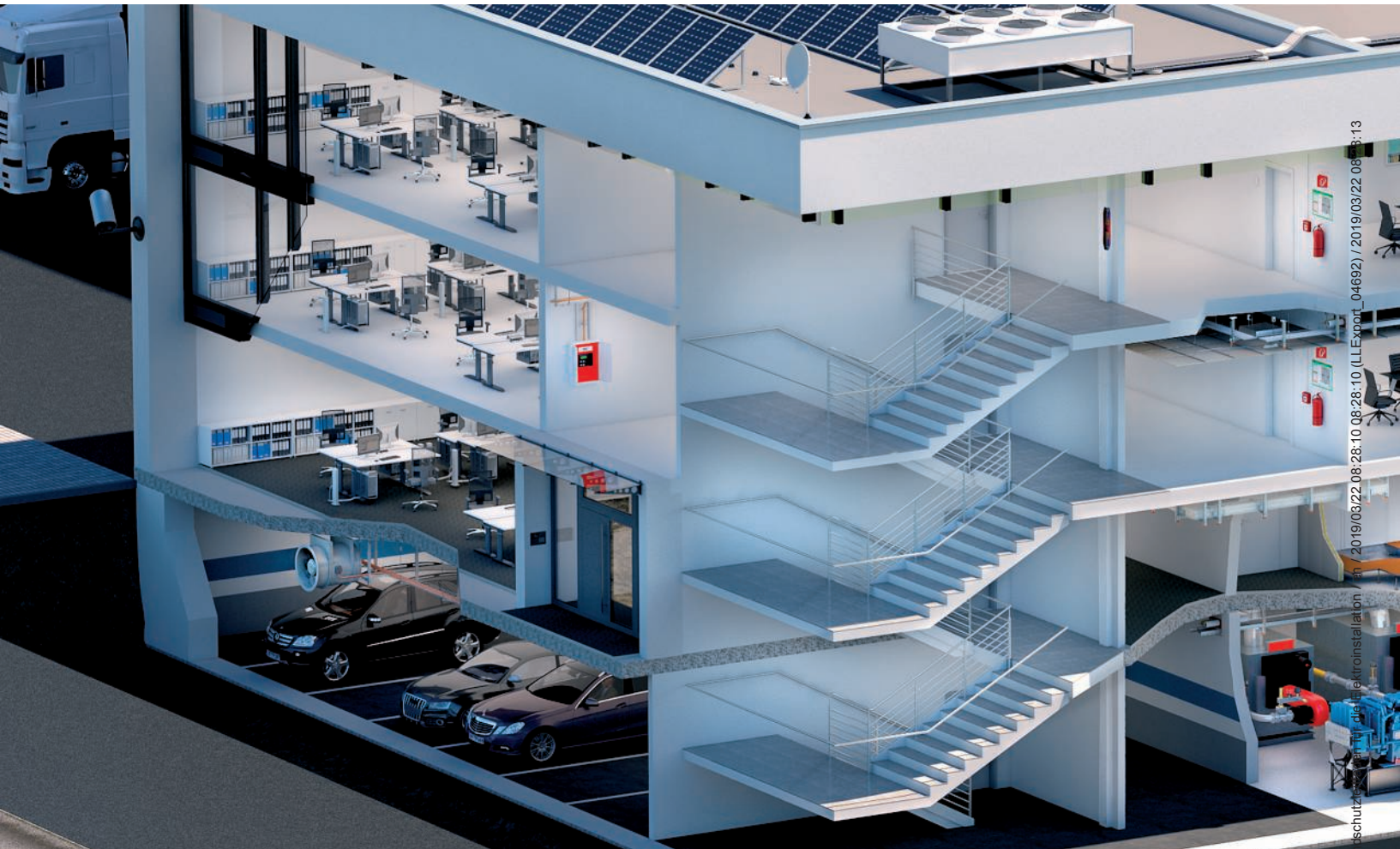
The formation of fire sections through firewalls or components with fire resistance
