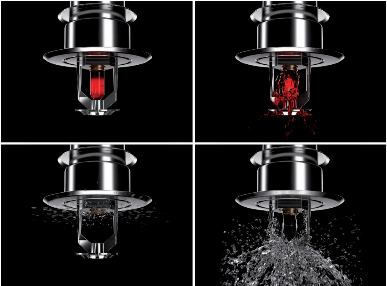
Triggering of a sprinkler head when a nominal temperature of 68 °C is exceeded on the glass vial
